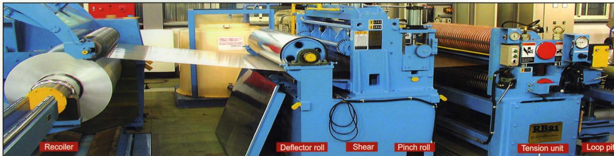
Typical layout of slitter line (recoiling part)
